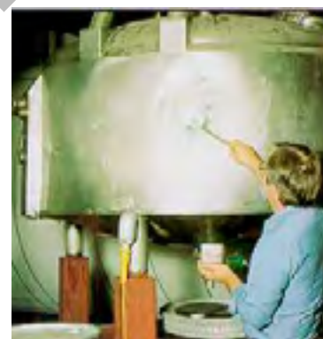
Stainless Steel Putty is ideal for making non-rusting repairs to stainless steel food processing equipment.
