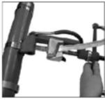
5. Roll tool over buckle, backing off with tension handle throughout entire rolling operation. Failure to back off with tension handle through-out entire course of roll-over may result in breaking of band. There is no loss of tension as band released is used up in
