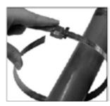
1. Band may be used from bulk roll as this completely eliminates waste of band. Slide buckle on band as shown, bringing end of band around object to be clamped and again through buckle. NOTE: The tension screw thread should be lubricated regularly.
