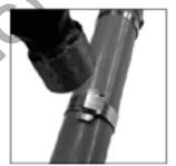
8. Hammer down buckle ears to hold band stub in place to complete BANDIT
