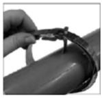
2. Continue band around object once more and again through buckle. Double banding develops a great deal more radial compression than single banding. Bend end of band under buckle.
